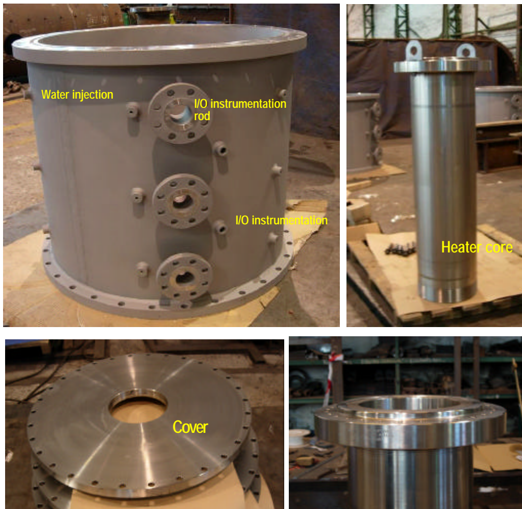
Figure 2-1: Main parts of the structure: external cylinder, heater core,annular cover and heater flange.
