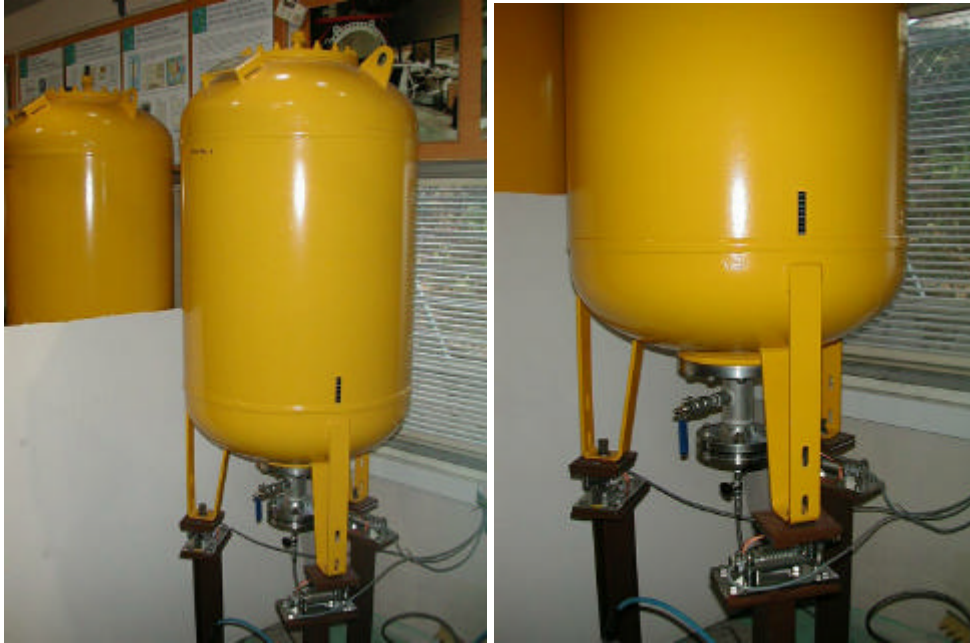
Figure 2-2: Hydration system: accumulator vessel and detail of the load cells.
