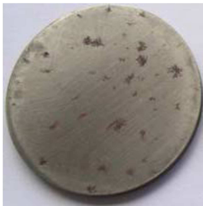
Figure 11. Photograph of the pitted surface of the steel plate after 22-month exposure to unsaturated compacted bentonite
