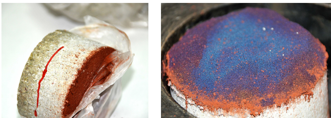
Figure 15. Photograph taken after the dismantling of the 52-month medium cell: (left) bentonite surface; (right) corroded iron powder.
