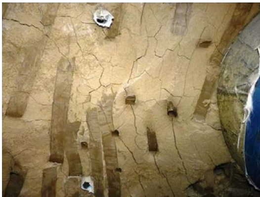
Figure 11: Drying of bentonite (after 5 days) and plastic for protection
