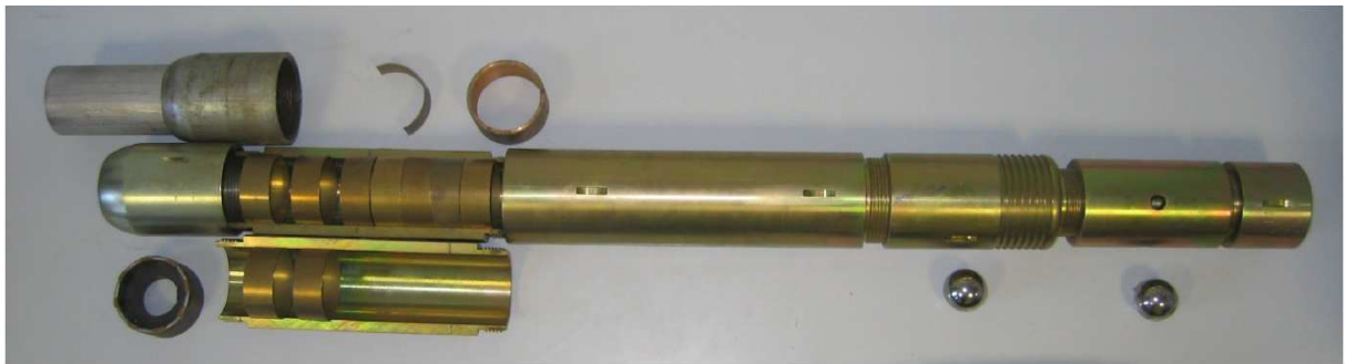
Figure 13: Ring sampler with thin wall prolongation
