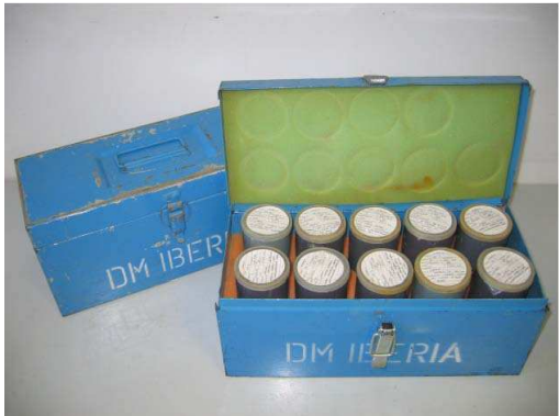
Figure 17: Transport box for samples (made in metal and with foam protection)
