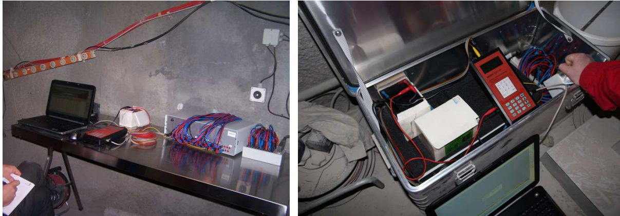
Figure 4: Pictures of the experimental setup; left: test measurement, laptop controlled; right: installation in an aluminum box for monitoring, device controlled
