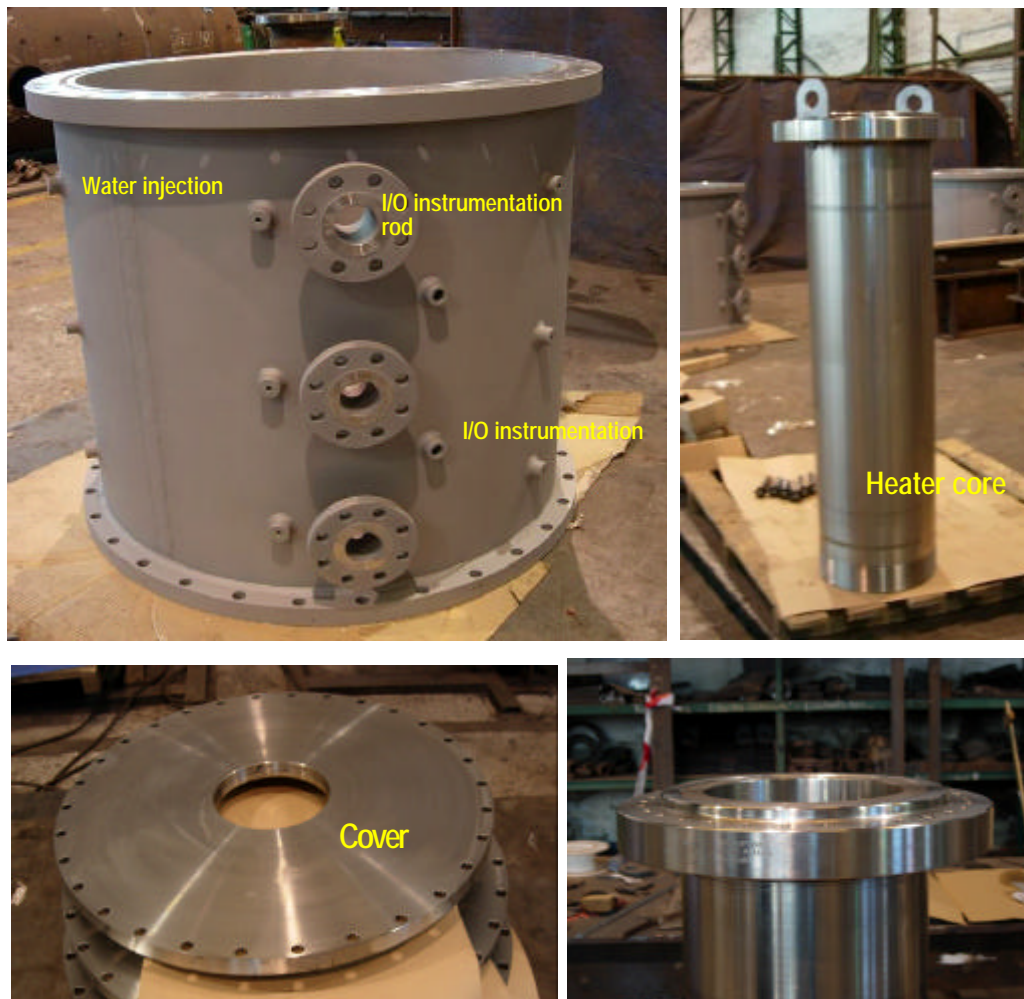
Figure 2-2: Main parts of the structure: external cylinder, heater core,annular cover and heater flange.
