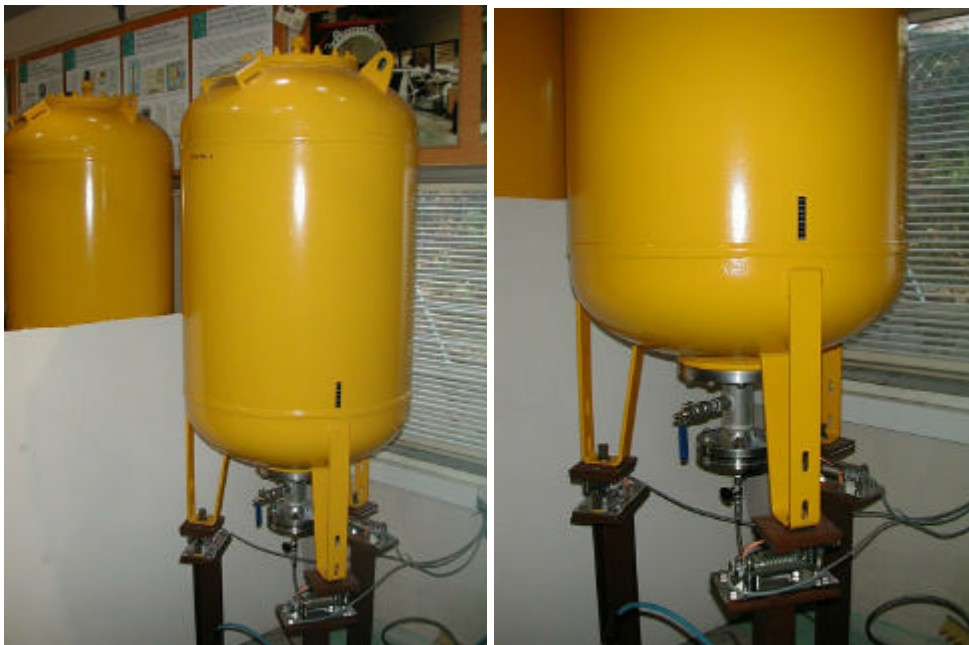
Figure 2-3: Hydration system: accumulator vessel and detail of the load cells.
