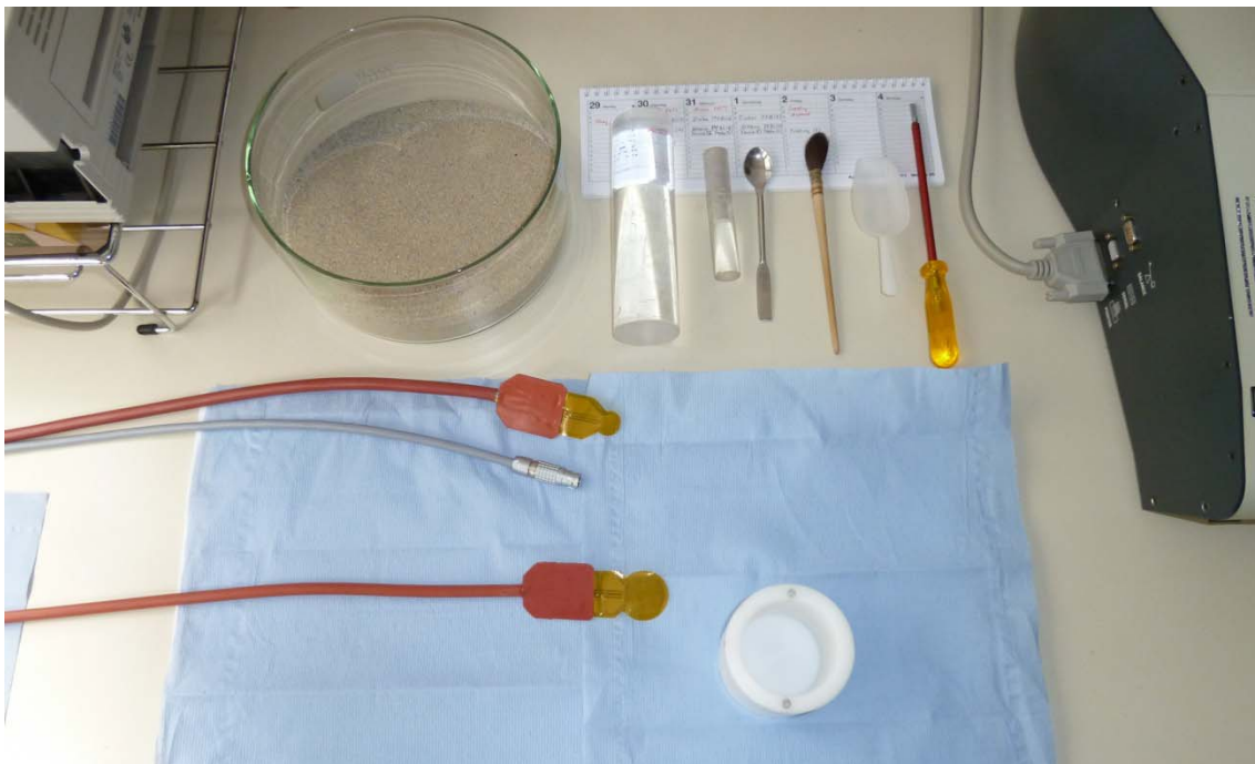
Fig. 2.2 Sensors for the Hotdisk analyser
