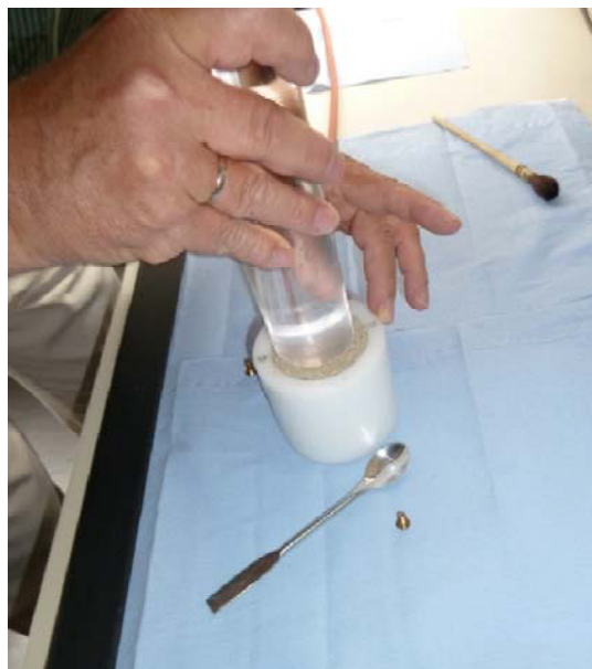
Fig. 4.5 Emplacement of second SB layer into the sample container
