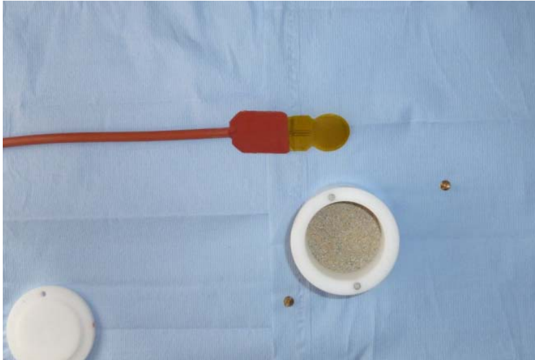
Fig. 4.2 Sample container with SB layer, in red: measurement sensor
