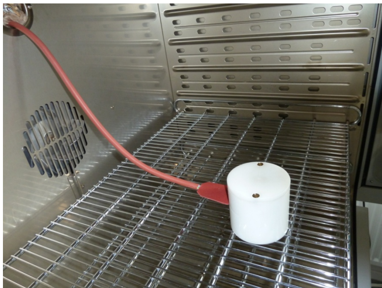
Fig. 4.7 Prepared sample in the oven
