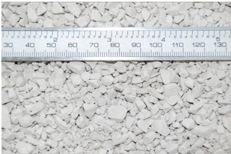
Figure 8 Crushed pellets used to fill the space between bentonite blocks and steel tank walls.
