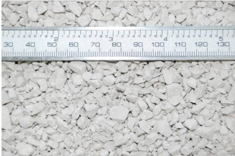
Fig. 2 Crushed pellets used to fill the space between bentonite blocks and steel tank walls.
