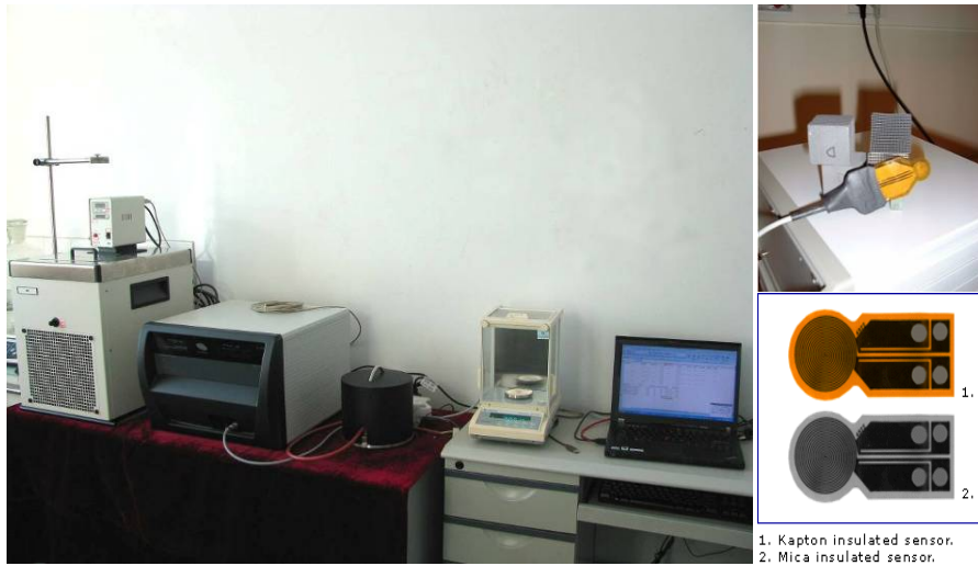
Fig. 3 Hot Disk thermal constants analyser and sensors.
