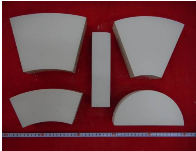
Fig. 1 compacted bentonite blocks.
