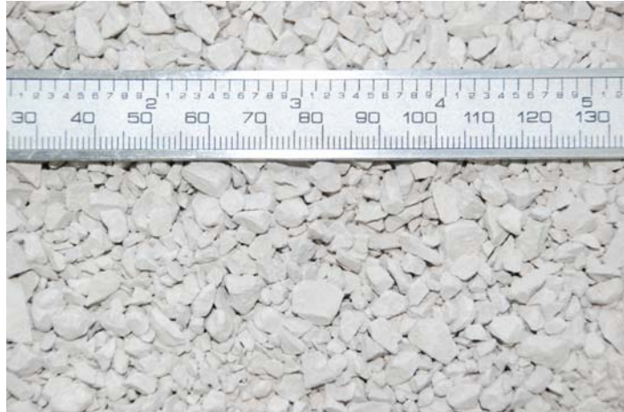
Fig. 3 Crushed pellets used to fill the space between bentonite blocks and steel tank walls.
