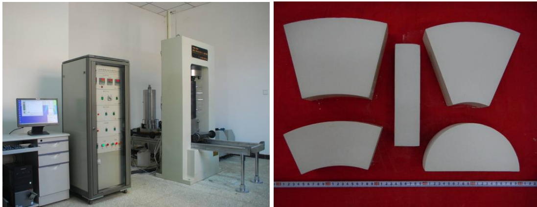
Fig. 2 Compressive test machine and compacted bentonite blocks.
