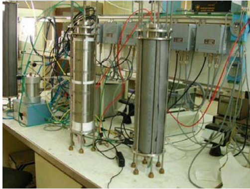
Infiltration cells in operation: isothermal (left) and with thermal gradient (right)
