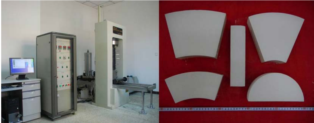
Figure 13: Compressive test machine and compacted bentonite blocks.
