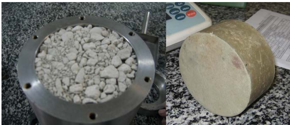
Figure 3: Appearance of the EB mixture after compaction and of the specimen after saturation.
