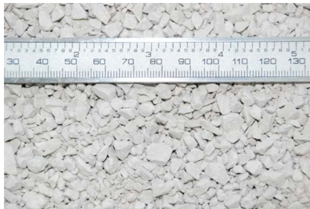
Figure 14: Crushed pellets used to fill the space between bentonite blocks and steel tank walls.
