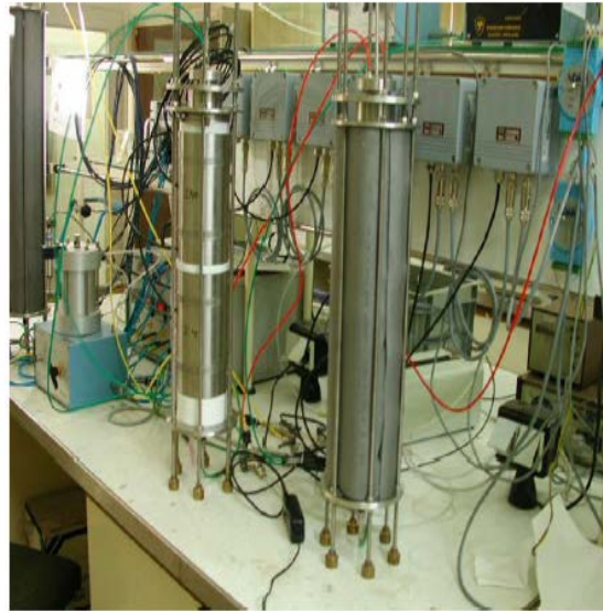
Figure 17. Infiltration cells in operation: isothermal, I40 (left) and thermal gradient, GT40 (right) (Villar and Gómez-Espina, 2009).
