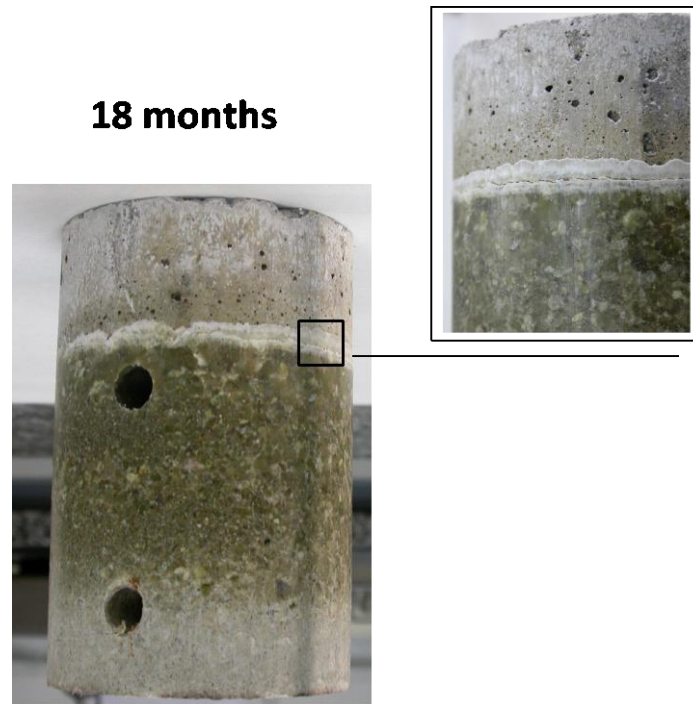
Figure 3. Photographs of the compacted bentonite block and the concrete slab after the dismantling of the 12 and 18-month tests
