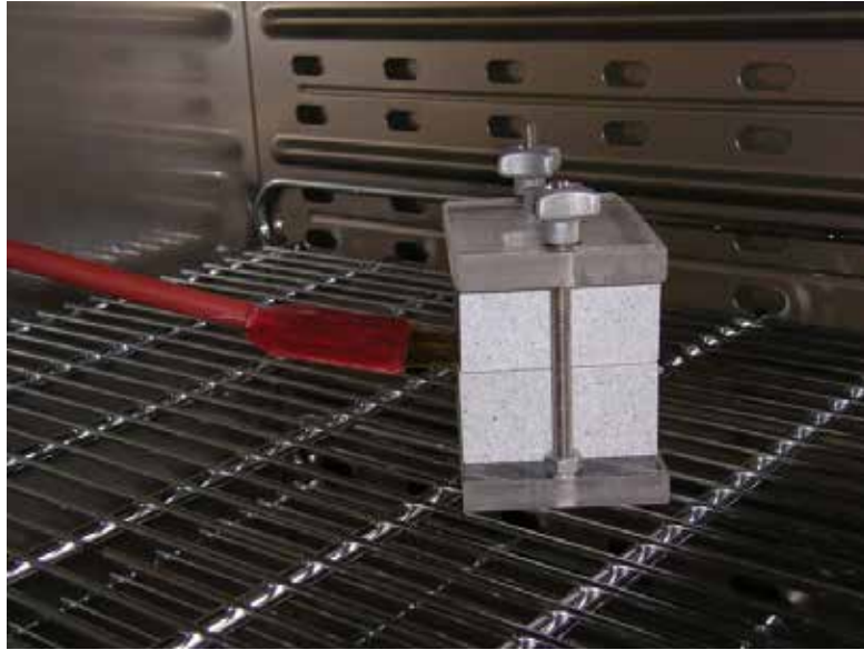
Fig. 3.3 Sample pair in the drying oven (the clamping device is used to assure coupling of sensor to the bentonite)
