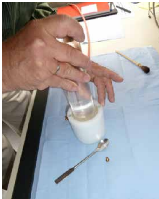
Fig. 4.5 Emplacement of second SB layer into the sample container
