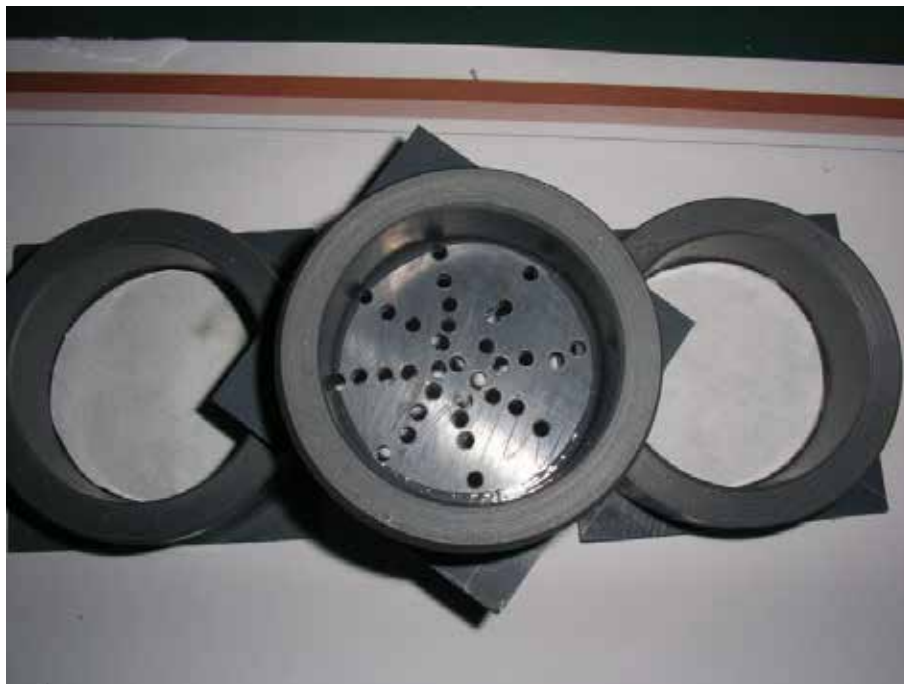
Fig. 4.13 PVC cell before placement of the sand-bentonite sample
