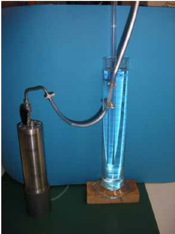
Fig. 4.17 System for measurement of sand-bentonite permeability to gas (left) and water (right)
