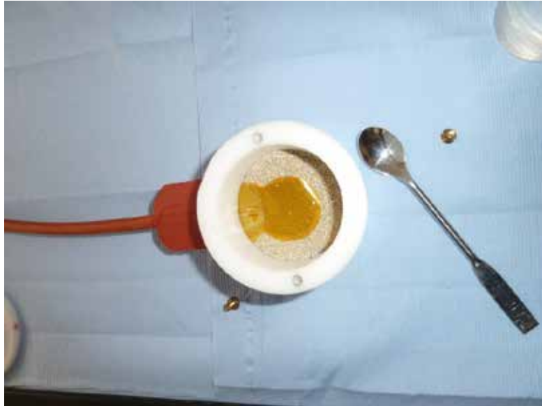
Fig. 4.4 Sensor and SB layer inside the sample container
