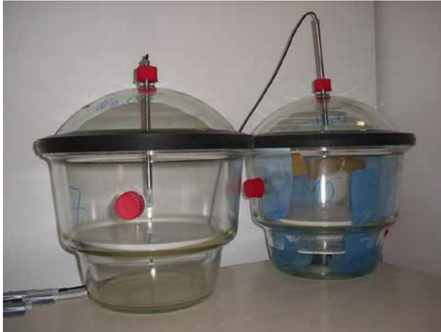
Fig. 4.12 Exsiccators with sensors for temperature and humidity measurement
