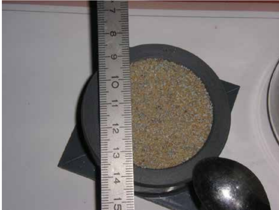
Fig. 4.14 Measurement cell filled with sand-bentonite sample
