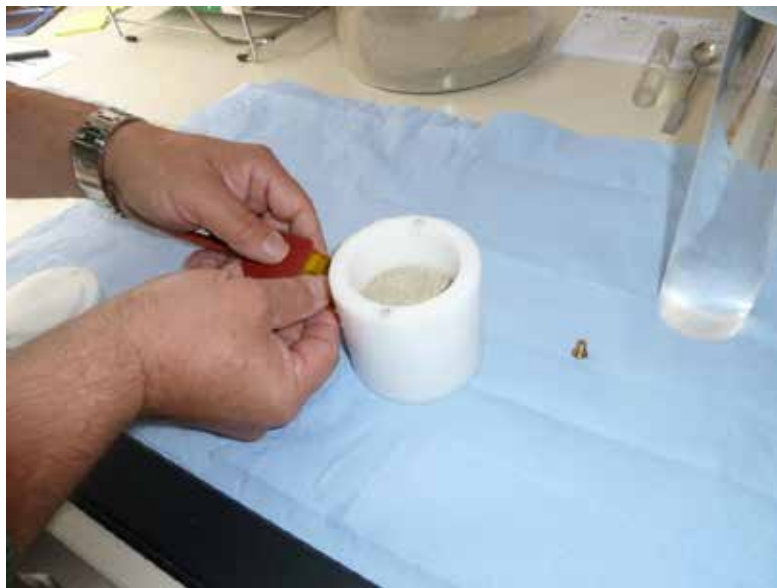
Fig. 4.3 Inserting the sensor into the sample container
