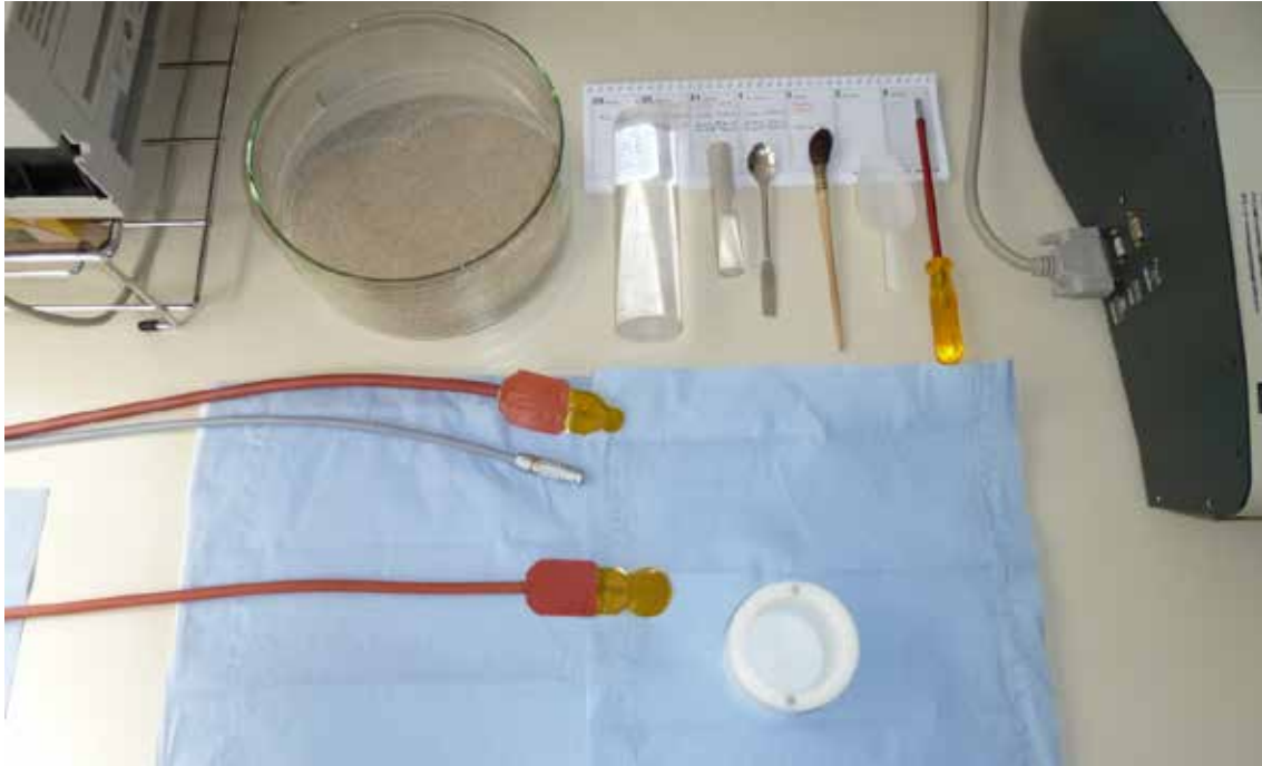
Fig. 2.2 Sensors for the Hotdisk analyser
