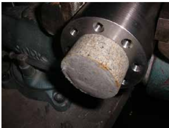
Fig. 4.18 Removal of saturated sand-bentonite from the cell
