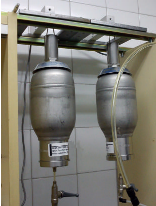
Figure 13: Water deposits and load cells
