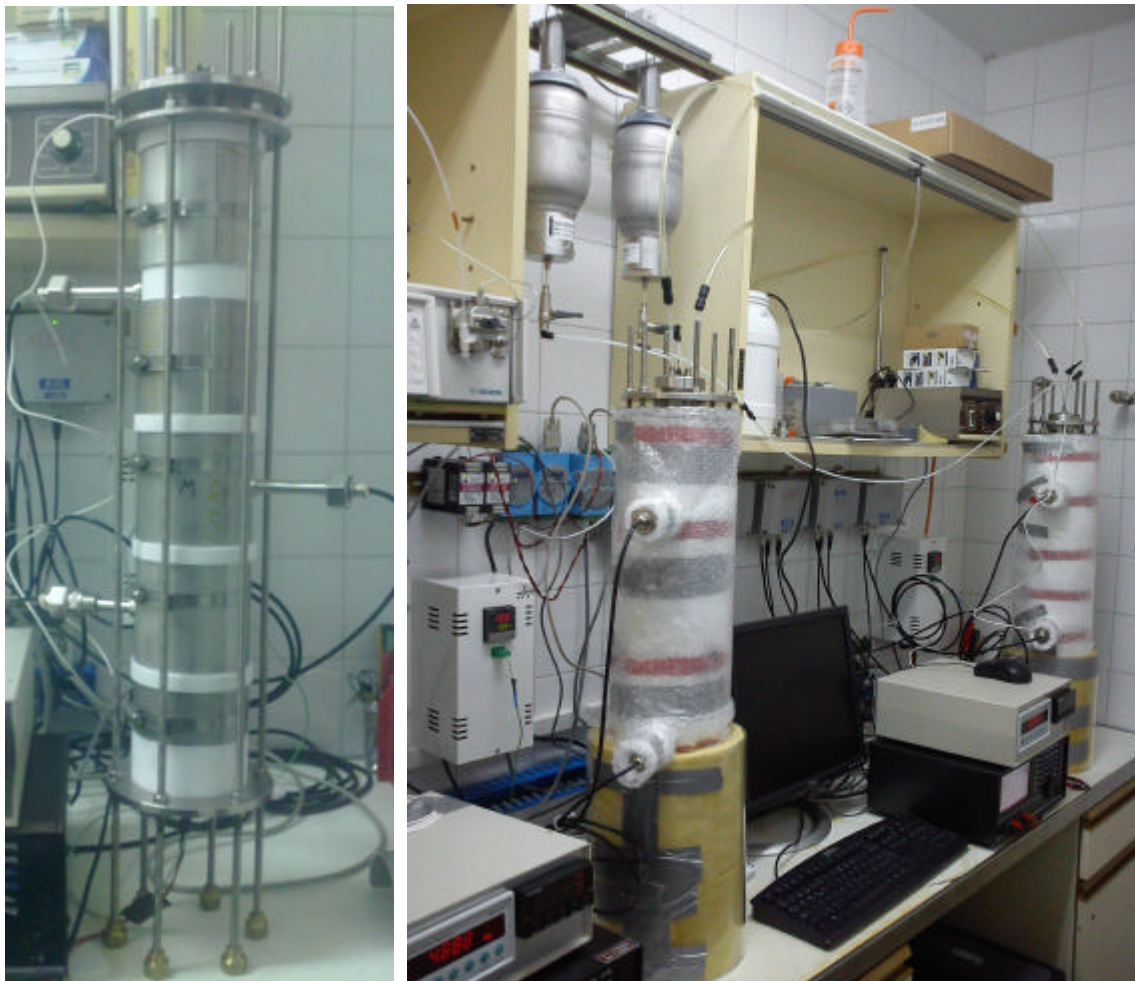
Figure 19: Cell B before being wrapped with the insulation material (left) and THM cells in operation (right)
