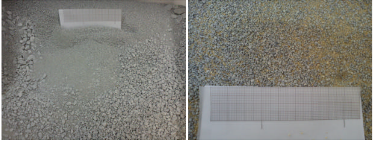
Figure 2: Appearance of the materials received at CIEMAT: MX-80 pellets (left) and sand/bentonite mixture (right)
