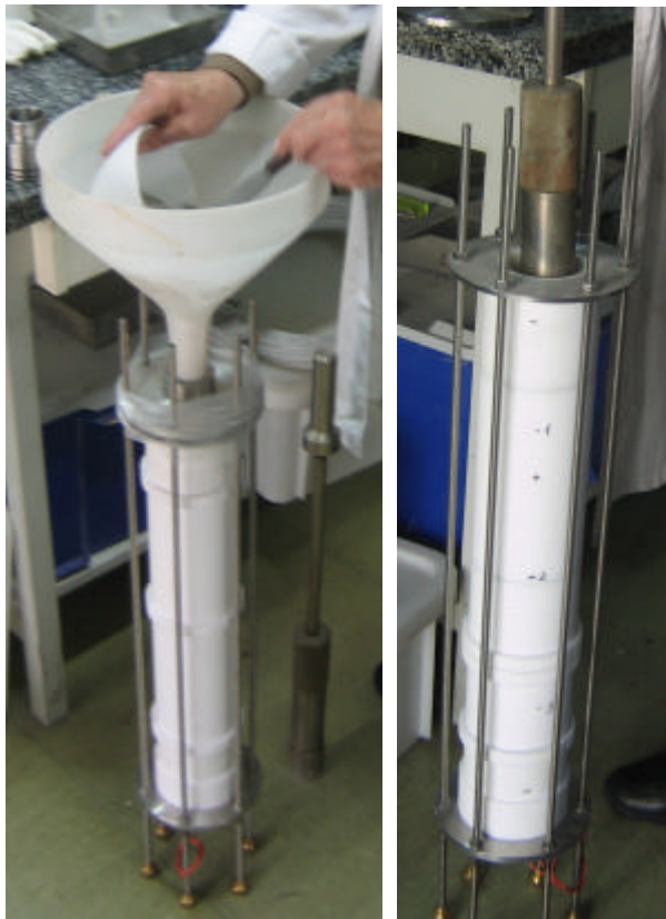
Figure 17: Pouring of the pellets granulate inside the cell (left) and compaction of the S/B mixture (right)
