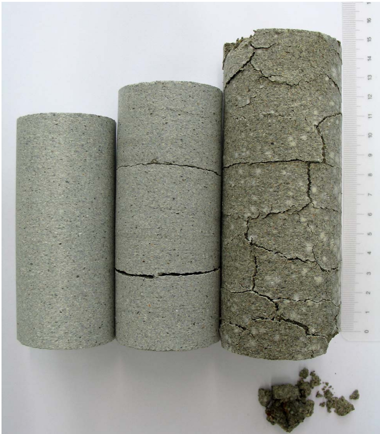
Fig.2: Cores from the bentonite block stored at different relative humidity for 6 months. Left ambient condition (50-60% r.H.), middle 75% r.H., right 99% r.H.
