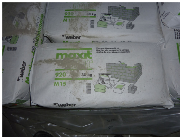
Fig. 3.15: Cement mortar type M15 (Maxit 920)
