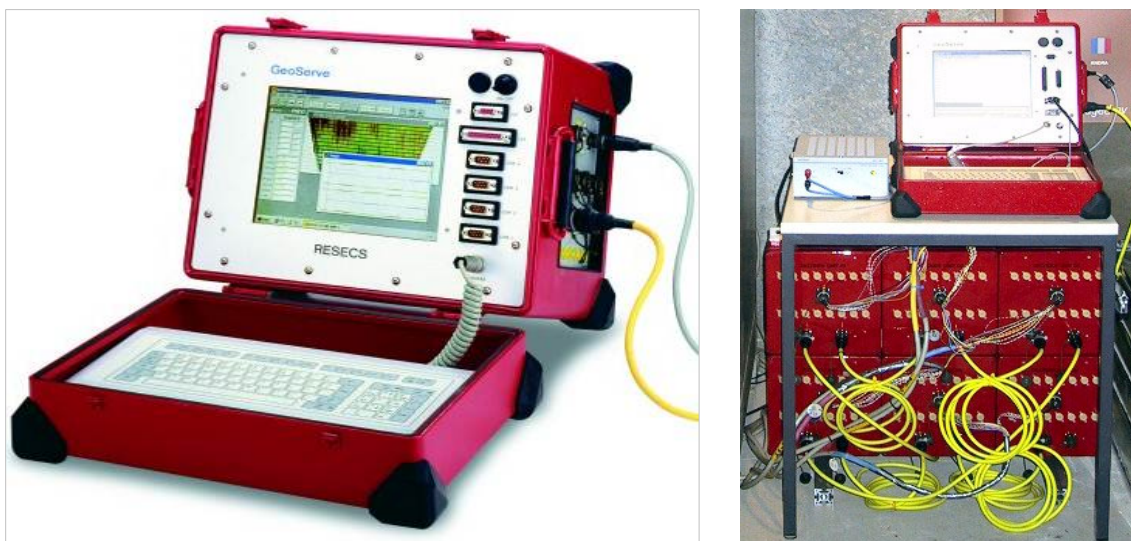
Fig. 5.31: RESECS measuring system (left) and decoder boxes (right).
