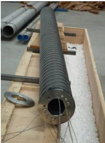
Photographs 4.3.1 and 4.3.2: Heater central tube with the resistors cables around it. Detail of the exit of an internal thermocouple.
