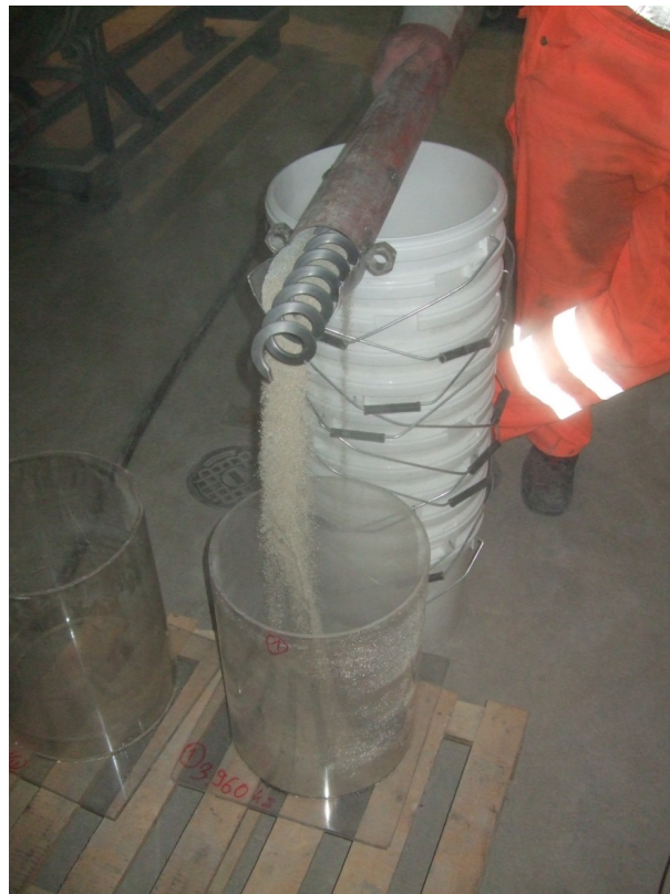
Fig. 6.26: Sand/bentonite sample preparation.
