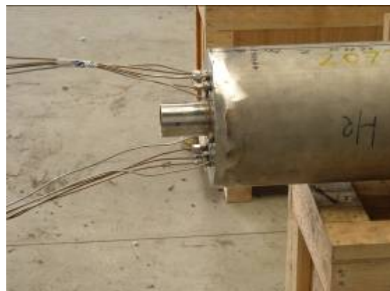
Photographs 4.3.5 and 4.3.6: Details of heater 2 back and front lid after welding.
