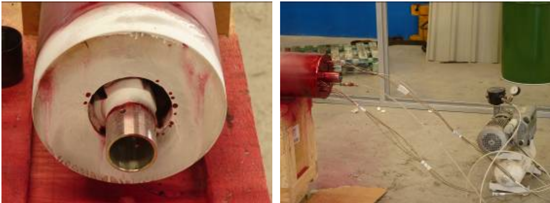
Photographs 4.3.7 and 4.3.8: Qualification of the welding with dye penetrant inspection test and flushing operation.
