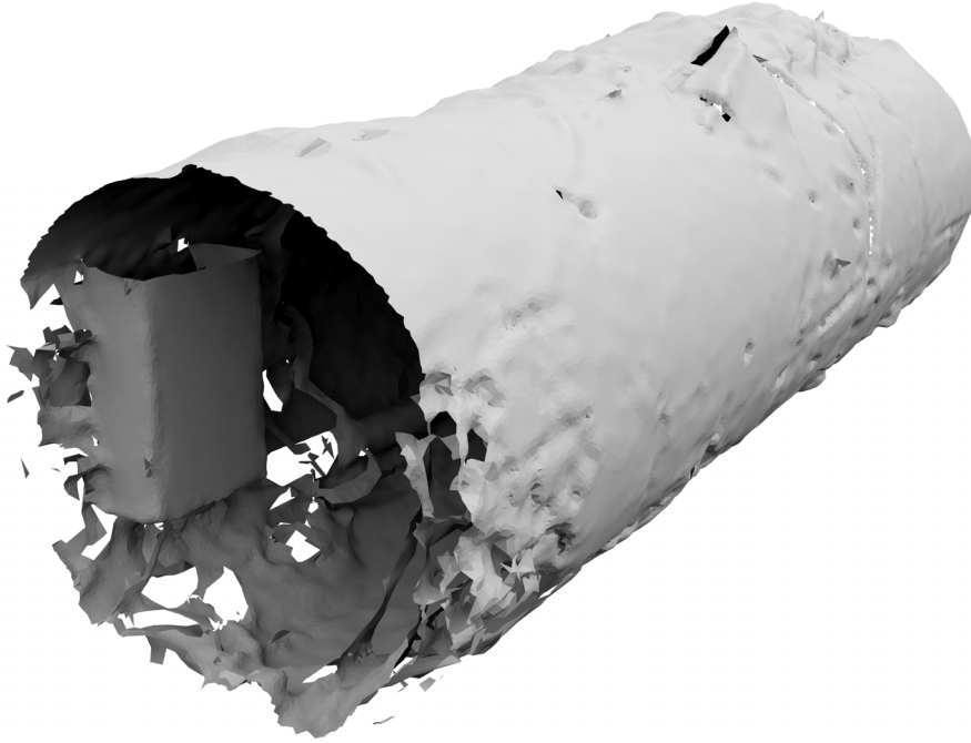
Fig. 6.20: Laser scan of the sand/bentonite section (TM HE-E 27.18 - TM HE-E 31.18)
