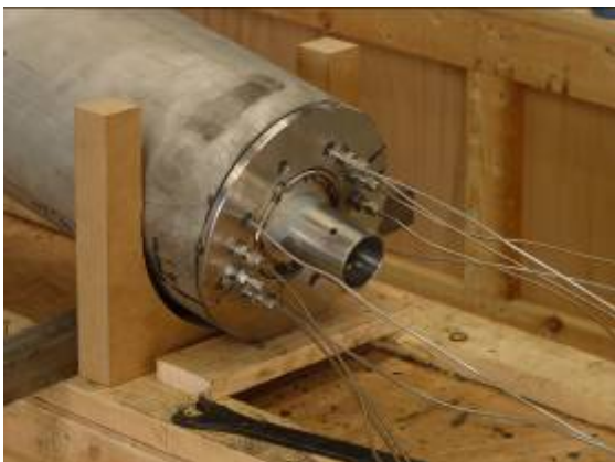
Photographs 4.3.3 and 4.3.4: Insertion of the central tube inside the outer protection tube. Detail of heater 2 front lid before welding.
