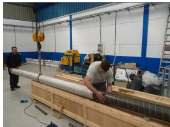
Photographs 4.3.3 and 4.3.4: Insertion of the central tube inside the outer protection tube. Detail of heater 2 front lid before welding.
