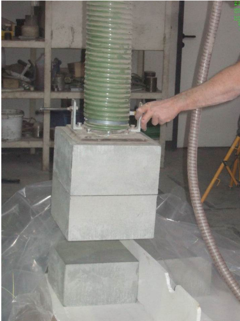
Fig. 3.3: Sticking capacity of two bentonite blocks by moisturing the connected surface (provided by Alpha Ceramics, Germany).
