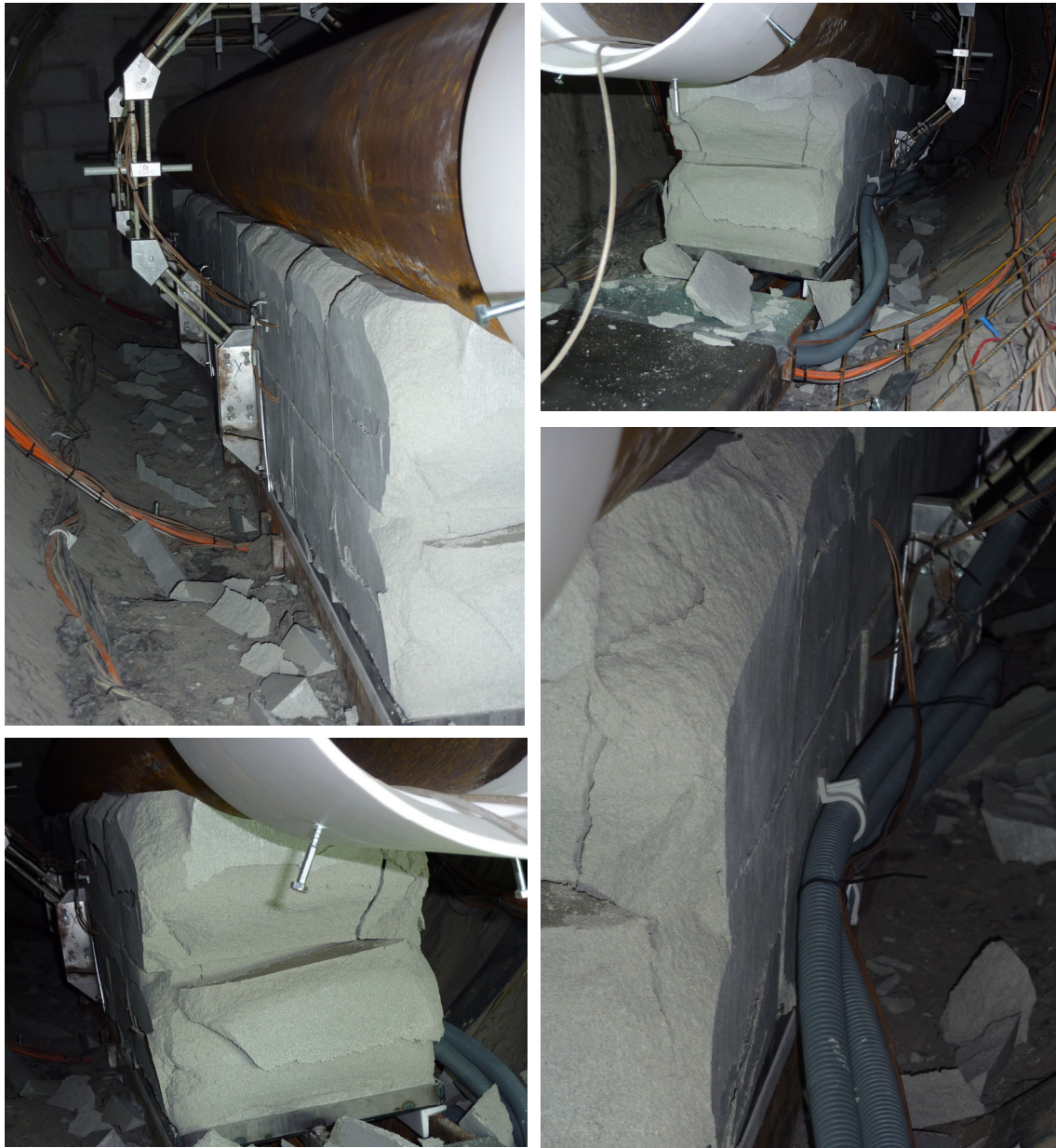
Fig. 6.14: Failure modes of bentonite blocks.
