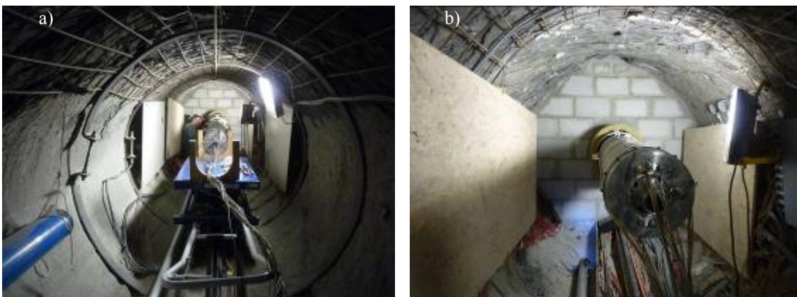
Fig. 6.30: a) Heater 2 at the liner entrance; b) Heater 2 partially introduced inside the liner.
