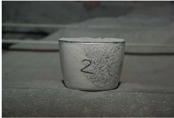
Fig. 3.13: Segregation observed in a glass bowl placed onto the progressing slope of the filling material
