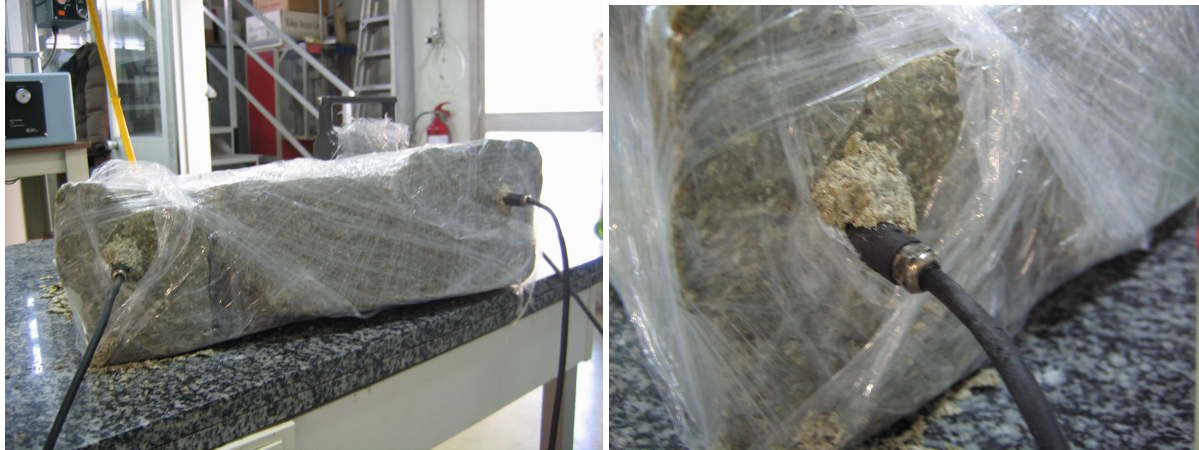
Figure 8: Insertion of capacitive sensors in blocks for measurement of RH and T
