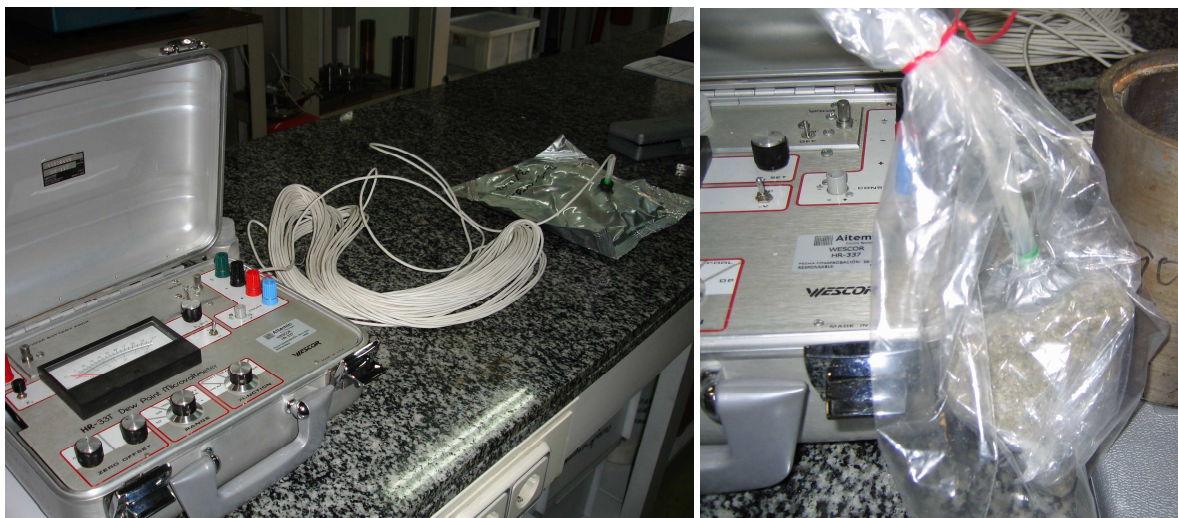
Figure 9: Measurement of relative humidity and temperature with psychrometers
