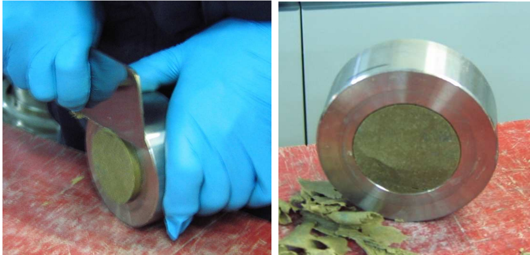
Figure 13: Preparation of a sample for permeability determination
