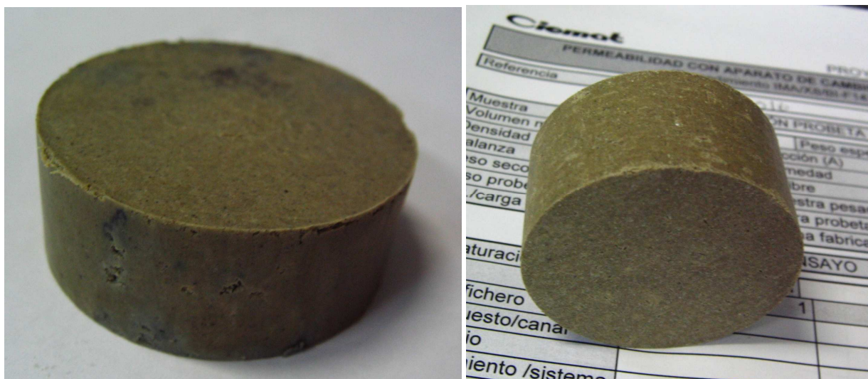
Figure 29: Appearance of B-S samples after the permeability tests
