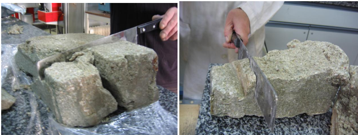
Figure 9: Sectioning of blocks to obtain subsamples
