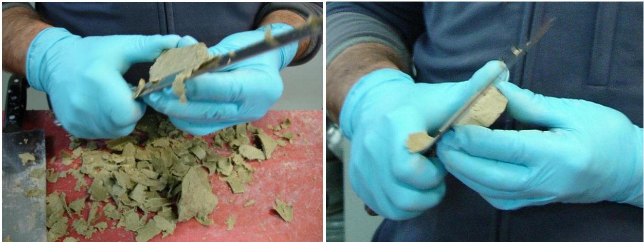
Figure 8: Trimming of a sample in the laboratory for water content and dry density determination
