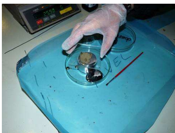
Use of mercury to determine the volume of the subsamples
