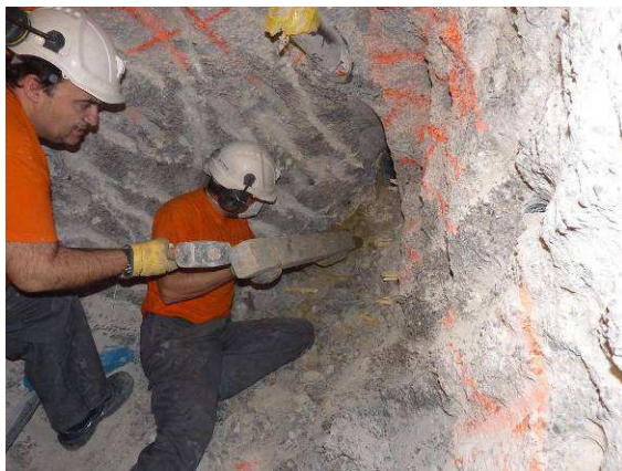
Hammering the sampling pipe into the bentonite
