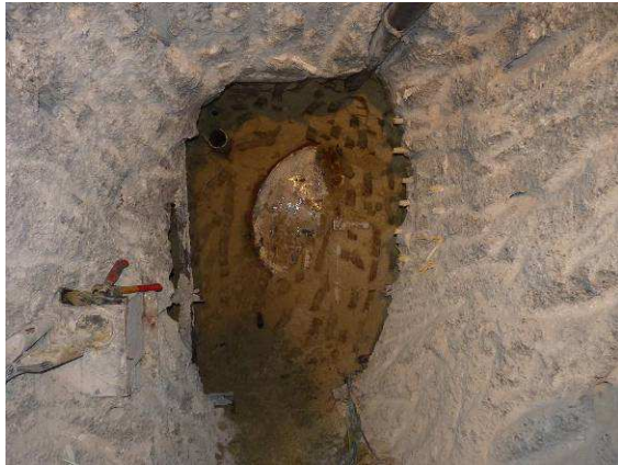
Front face of the canister. A layer of around 75 cm of bentonite already removed
