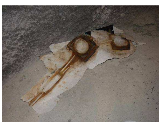
Geotextile covering total pressure cells
