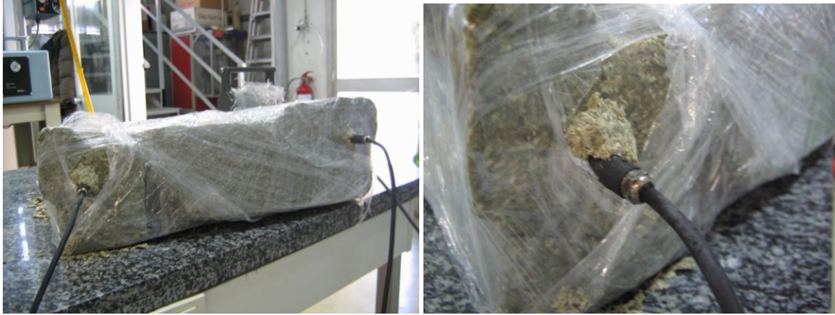
Figure 10: Insertion of capacitive sensors in blocks for measurement of RH and T
