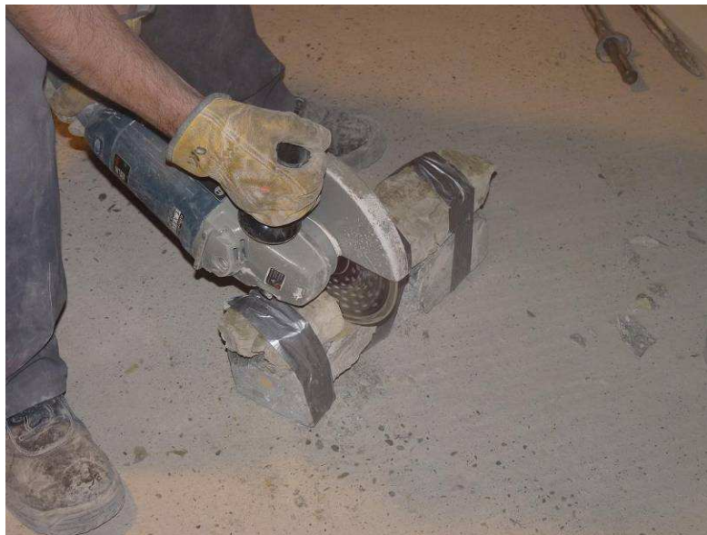
Preparing concrete/bentonite interface samples by cutting them
