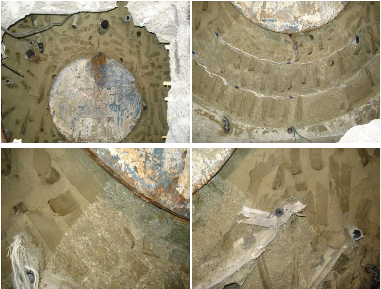
Figure 3: Appearance of the GBM (left up), the bentonite blocks (right up), and the GBM-blocks contact (bottom) upon dismantling.
