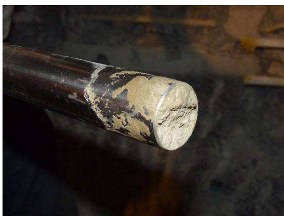
Bentonite sample inside the pipe
