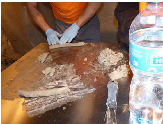
Preparation of the solid expansive cement
